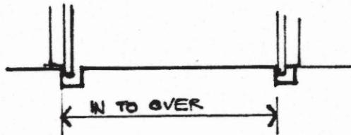
Lock the wheels on with a bit of Locktite 601. Squeeze the 'W'iron frames in a bit, so when you put in the wheels, they have to be sprung in.
