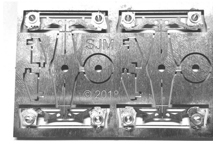
Image 1. Archbar bogie etch showing correct orientation of the waisted bearings. Tabs on the angle brackets can be twisted with pliers to secure the parts prior to soldering.
