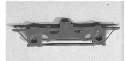
Image 2. Flash has been trimmed from the sideframe casting and holes have been drilled to clear the waisted bearings that protrude from the bogie frame.
