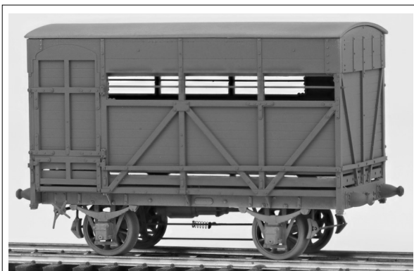
Photo 8. Side and end bracing.
