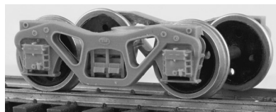
Photo 3. Flash has been trimmed from the sideframe casting and holes have been drilled to clear the waisted bearings that protrude from the frame.
