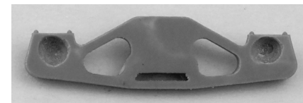
Photo 3. Holes are drilled in the back of the sideframe so it fits over the waisted bearings protruding from the frame.
