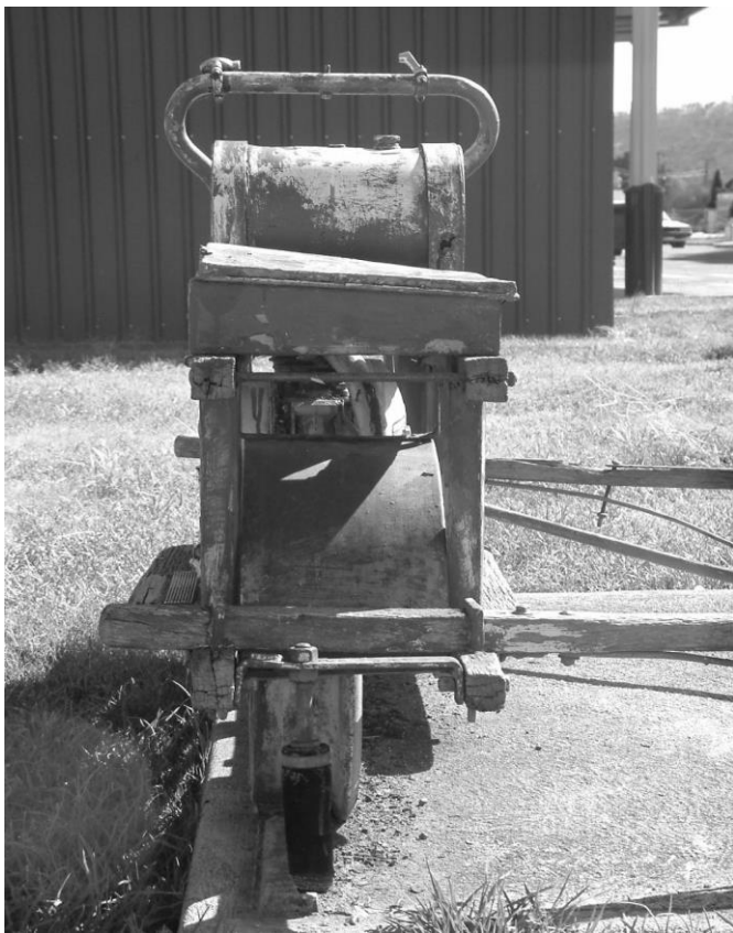
Photo 1. The wheel is offset in the body. Note how the mudguard fills the full inside of the body.
