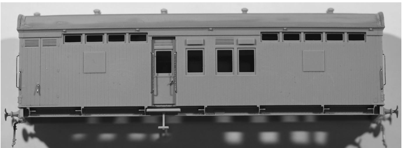
BOTTOM: Arrangement of the door handles, hand rails and the step below the door on the side of the van. Note the centre roof vent sits above the storage compartment at one end of the van.
