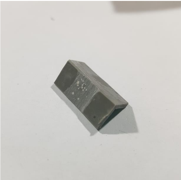
Figure 7, right angle with notch filed out
