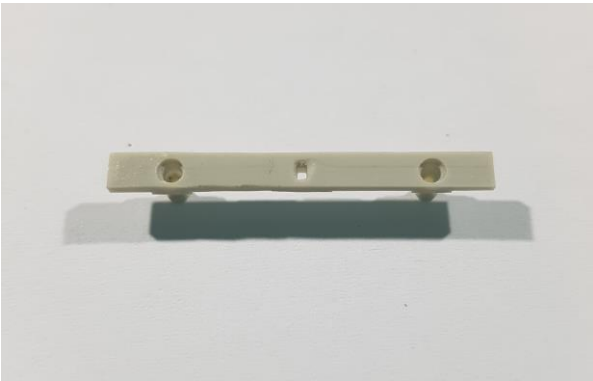
Figure 2, head stock showing drilled holes
