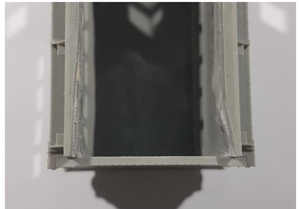
Figure 6, insides of BKD solebars filed back for springing
