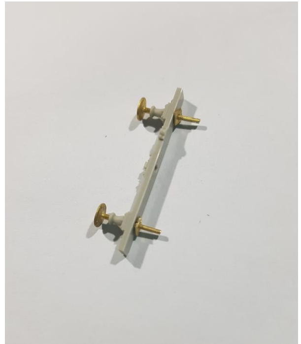
Figure 4, fitted buffers with stoppers soldered
