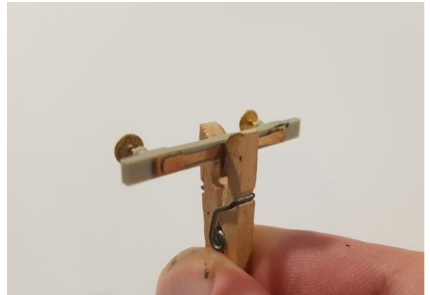
Figure 5, peg holding spring in place while glue sets
