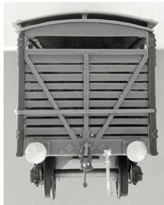
Image 5. End view showing location of horizontal bars and brake hose.
