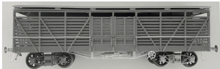
Image 4. Side view of an 1895 wagon showing the location of the horizontal bars, the brake wheel and locking handle.
