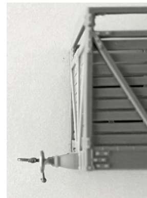
Image 6. Adjust the position of the hook so that the turnbuckle on the coupler lines up with the faces of the buffers.
