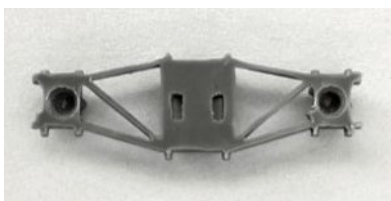
Image 8. Flash has been trimmed from the sideframe casting and holes have been drilled to clear the waisted bearings that protruding from the bogie frame.
