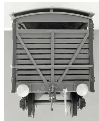
Image 4. End view showing location of horizontal bars and brake hose.
