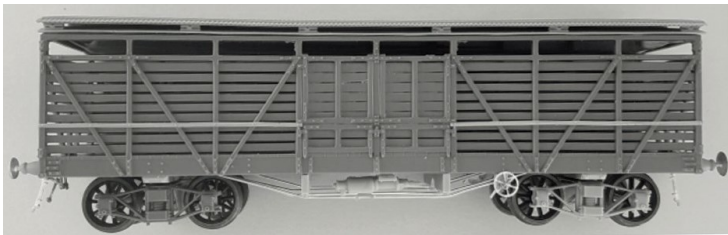
Image 3. Side view of an 1895 wagon showing the location of the horizontal bars, the brake wheel and locking handle.
